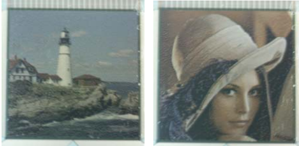
Figure 9 Two photographs taken of a mirasol display with a RGBY quad color tile
