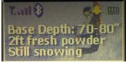
Figure 8. A photograph from a manufactured mirasol display with a RGB triad color tile
